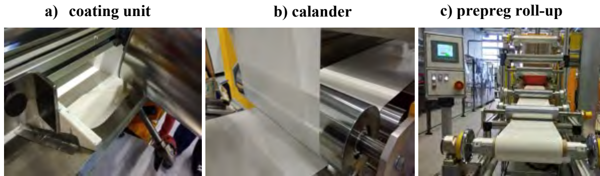
Figure 48 Detailed view of a) the coating unit, b) the calander, where the GF fabrics get impregnated with the resin formulation, and c) the prepreg roll-up for further storage.
