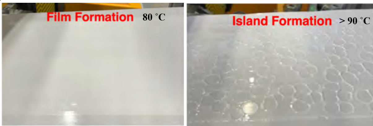
Figure 73a) Viscosities of EN and EN_Hybrid in dependency of temperature. b) A temperature of 80 °C at the coating head was determined to be optimal to reach a homogeneous film formation. Higher temperatures lead to a droplet „island“ film on the release paper.
