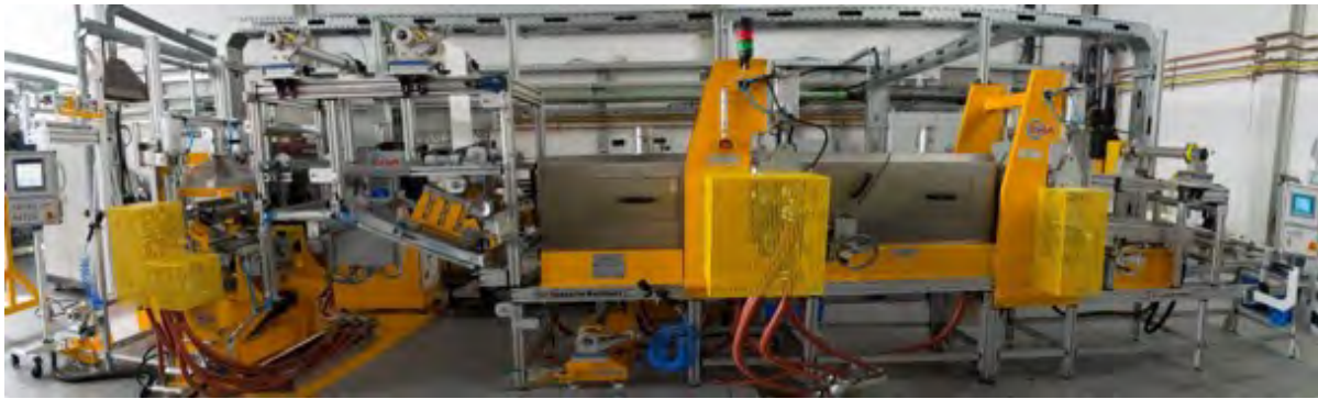
Figure 47 Lab-scale prepreg production on an EHA composites Machinery.
